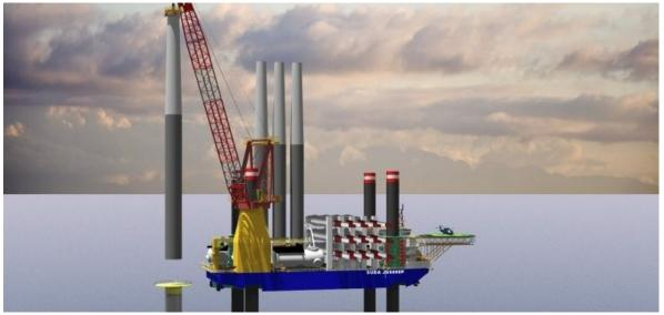
Suda's JG6000P is optimised for the offshore wind industry and can transport and install up to four 8 megawatt wind turbines
